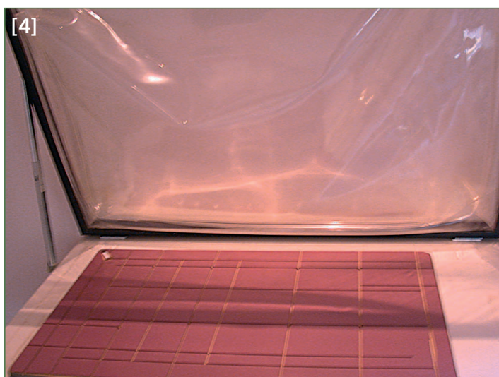
The plastic lid is vacuumed down over any object on the grooved sheet
