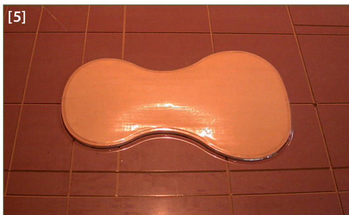
The plates are held together by the vacuum while the glue cures
