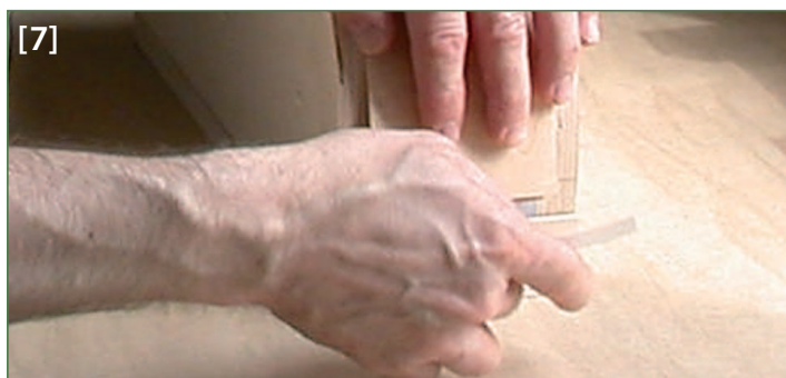
[7] The ends have to be wedged to the mould when fitting the rib sheets
