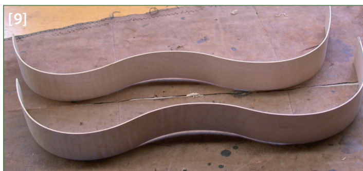
[9] The finished sheet is cut in half, producing two well-formed ribs
