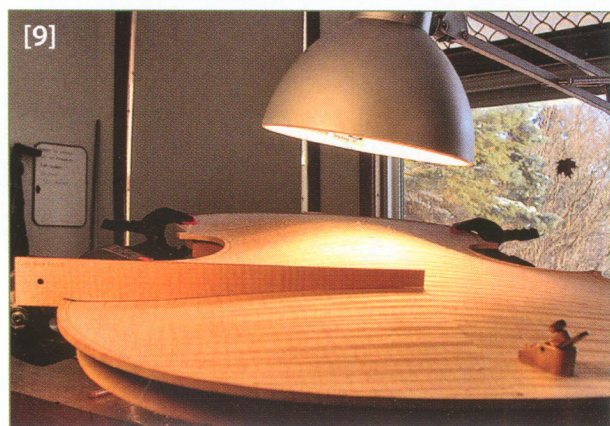
A cello template being used to shape a back
